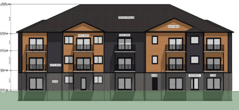
West Elevation/Façade ouest
